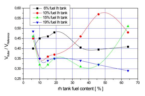
Figure 10: Flutter speed versus asymmetrical tank emptying.
