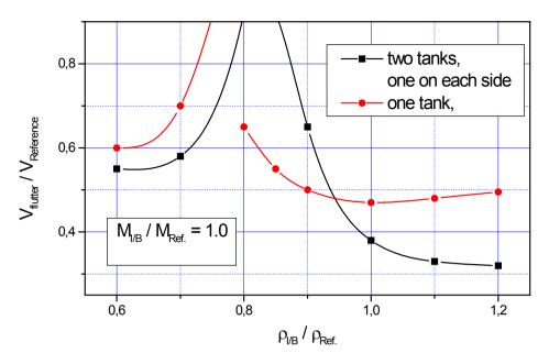
Figure 14: Flutter speed versus symmetric and asymmetric carriage, with radius of gyration variation.
