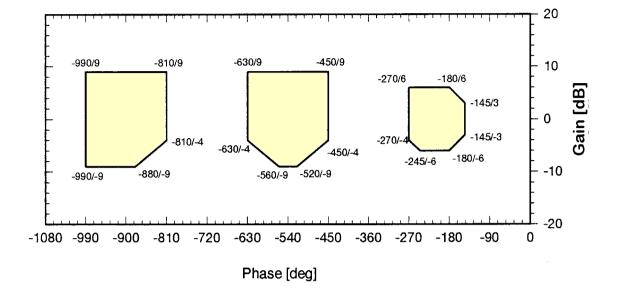
Figure 4: MIL-F-09490 Stability Margin Criteria for Open Loop Frequency Response Function.
