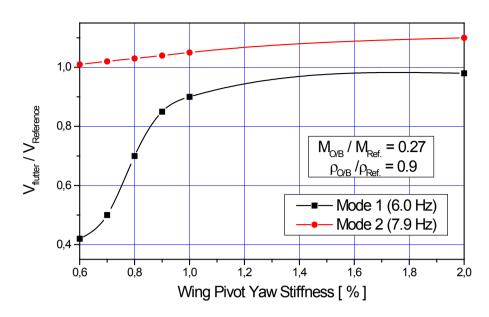
Figure 15: Flutter speed versus wing pivot yaw stiffness.
