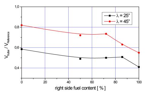
Figure 18: Flutter speed versus asymmetrical fuel emptying of Inboard tanks with symmetrical outboard stores.
