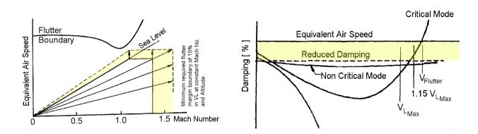
Figure 3: Graphical Representation of the Flutter Requirement MIL-A-8870.
