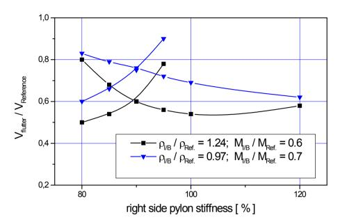
Figure 11: Flutter speed versus pylon stiffness.
