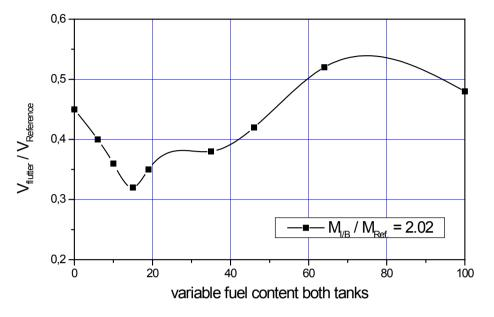
Figure 9: Flutter speed versus symmetrical tank emptying.
