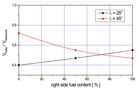
Figure 17: Flutter speed versus asymmetrical fuel emptying of Inboard tanks with symmetrical outboard stores.
